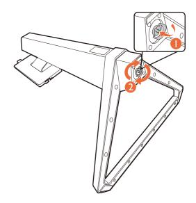
Orient and align the stand arm with the monitor, then push them together until they click and lock into place.
