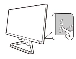
Turn on the computer too. If you have multiple video sources, press the looping key and the 5-way controller to select an input source.
