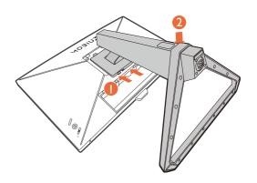
Carefully lift the monitor, turn it over and place it upright on its stand on a flat even surface.
